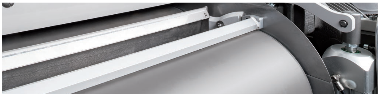
Sensor strip for roller temperature monitoring.
