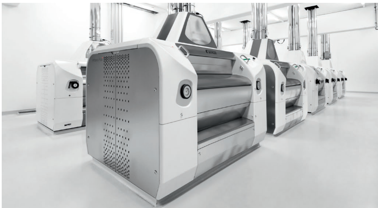
Antares Plus: Automatic grinding gap adjustment and temperature monitoring.
