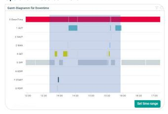
Operation modes are depicted in a Gantt chart, so you can specify the time period of interest. A scrutiny of the incidence before and after production stop can help you to reveal root causes.
