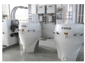
The Bühler dehuller: high throughput capacity and high oat dehulling degree.
