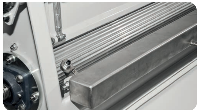
Fast cleaning thanks to easy access to the feeder and magnets.
