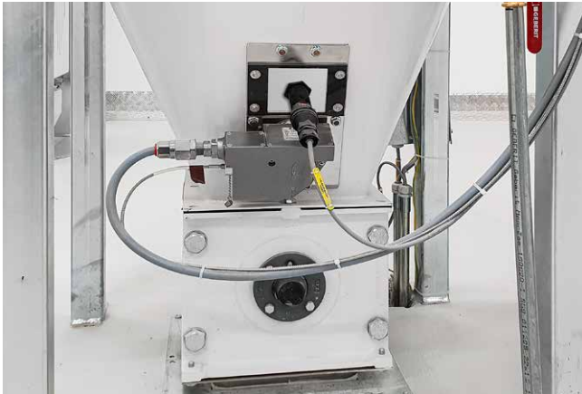
The compact NIR sensor head is suited to retrofit existing production plants.
